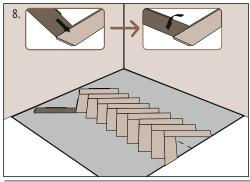
**Start with a new row,** find the 90 degree angle, connect the tongue with the groove, insert and fold down.
