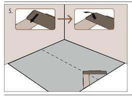
**Install the next plank** by inserting the tongue into the groove, adjust to a 90° angle and fold down. Press the top of the drop-lock joint down with the thumb to properly align the joint. You can use a rubber mallet to make sure the tongue and groove are properly clicked together. Keep the force used to a minimum.
