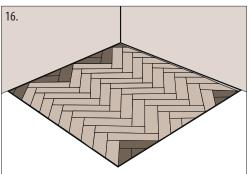
**Finish the installation,** all the planks shall be seamlessly connected, and the parquet pattern shall appear straight and symmetric.
