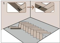
**Connect the next plank** by the short side: connect tongue with groove and fold down. Then connect the plank on the long side by pulling the plank towards you. If needed, use the rubber mallet and tapping block to firmly close the tongue and groove connection.
