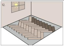
**The last plank of this row needs to be cut and adjusted** as previously done to the first plank at the beginning of the installation (see point 4).
