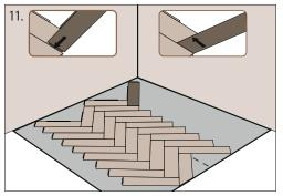
**Start with the next row,** connect the plank first by the short side. See step 9.
