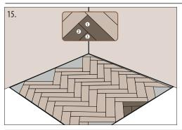
To fill the empty areas, measure carefully to find or cut the missing pieces. Start with the longest piece, then the shorter and end with the shortest.
