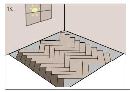
When installing the row beside the wall, always keep the necessary expansion gap (see table point 3.) from plank to the wall.
