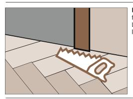
**Door frames** need to be undercut to allow for possible expansion of the finished floor under the door frames
