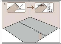
**Define the INSTALLATION LINE** to ensure the straightness. Place the first plank on the <u>center line</u> with its long side tongue facing upwards. Define the middle point of its short side, meet this point with the center line and build a 45° angle. The installation line runs through the top edge of the plank and is parallel to the center line.
