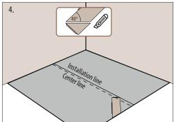
**Cut off a 45° equilateral triangle** from the lower part of this plank. Cut the boards decor side up. To cut, use a utility knife, move along the surface of the plank with even pressure and snap. Now place the cut side onto the boarder, keeping an expansion gap of 6mm min. (see table point 3. Before you start)
